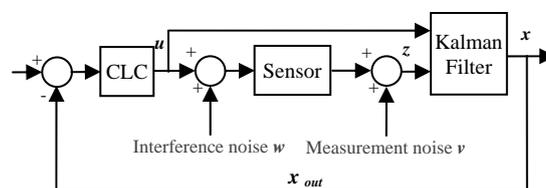
Figure 9. The CLC Structure based on Kalman Filter
