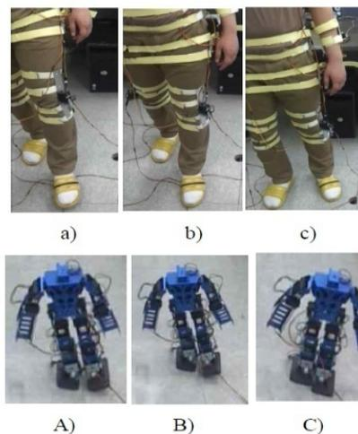
Figure 11. Static Walking of MS-robot
