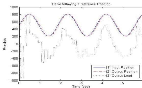
Figure 7. Servo Following a Reference Speed (CLC)
