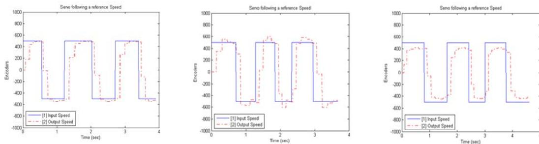
Figure 8. Effects of the Supplied Voltage (9v, 10.5v, 12v) to the Servos in the Outputs Velocity Response
