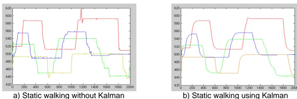
Figure 12. The Comparison of Robot Position Feedback for using or Not using Kalman Filter in Static Walking Control Experiment
