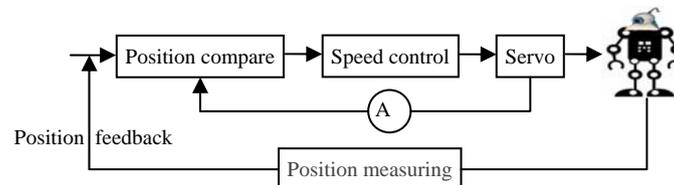
Figure 6. Close Loop Control Structure
