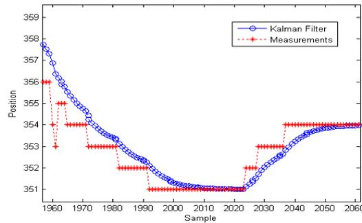
Figure 10. The Optimizing of Control Signal by Kalman Filter
