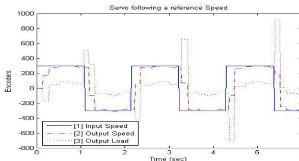
Figure 5. Servo Following a Reference Speed (OLC)
