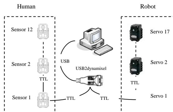
Figure 2. Man-Function Robot Control Structure
