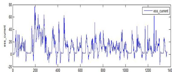
Figure 8. Current Profile Sampled during UDDS Cycles
