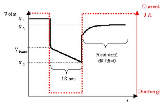
Figure 2. HPPC Test Profile
