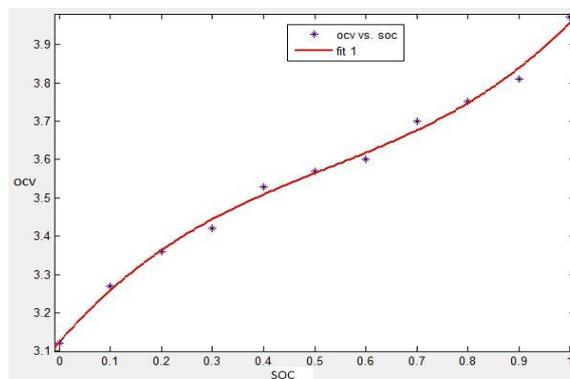
Figure 5. The Relationship between SOC and OCV After Fitting
