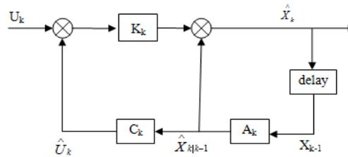
Figure 6. The EKF “feedback and calibration” Chart
