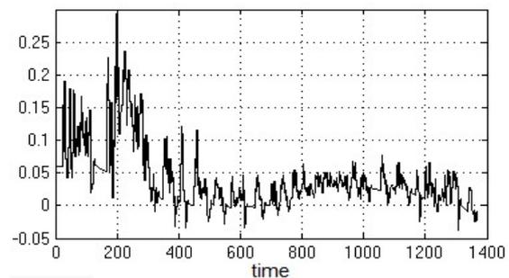
Figure 11. SOC Estimation Error Curves with EKF Algorithm
