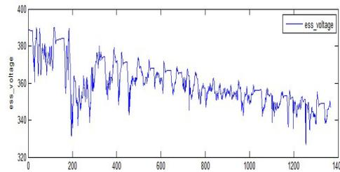
Figure 9. Voltage Profile Sampled during UDDS Cycles
