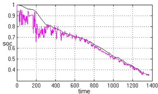
Figure 10. SOC Curves with EKF Estimation and Experiment
