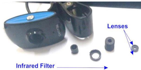
Figure 6. Internal component of web cam
