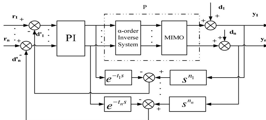
Figure 4. Block of DOB based on Pseudo-linearization System
