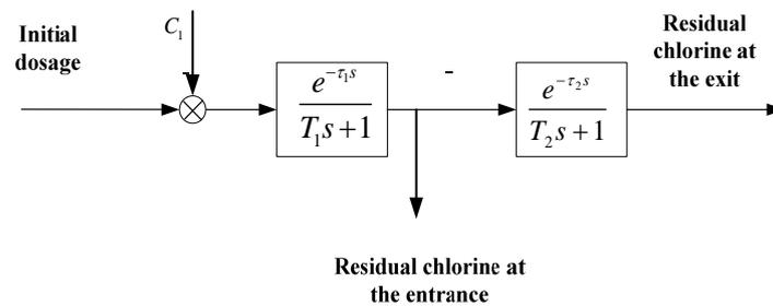
Figure 2. Single Tunnel Single Pool Chlorine Injection Process Model
