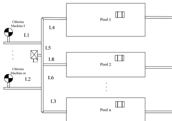
Figure 1. Multi Tunnels Multi Pools Structure Sanitizer Dosing System
