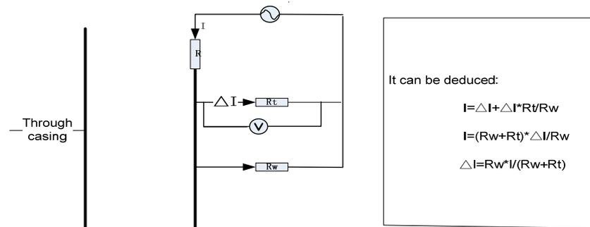
Figure 5. Improvement Model of the Precision Resistor Array
