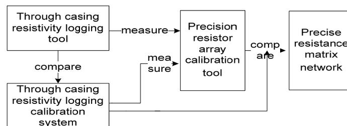
Figure 3. The Quantity Traceability System of Through-casing Resistivity Logging Tool
