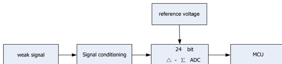
Figure 7. Acquisition System Design
