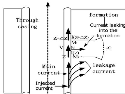
Figure 1. Principle of through Casing Resistivity Logging
