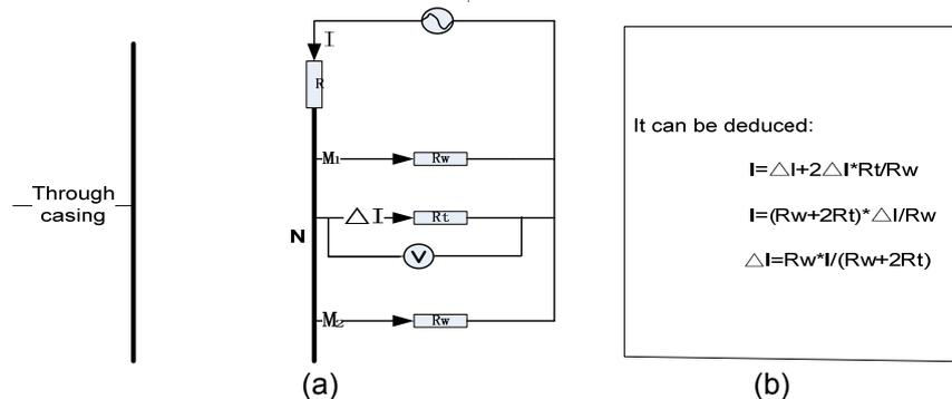
Figure 4. Precision Resistor Array Model
