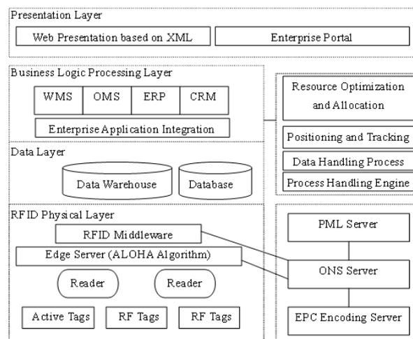
Figure 2. Integrated Real-time Management System Framework based on RFID
