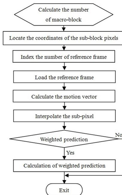
Figure 2. The Flow Chart of Inter Prediction Algorithm
