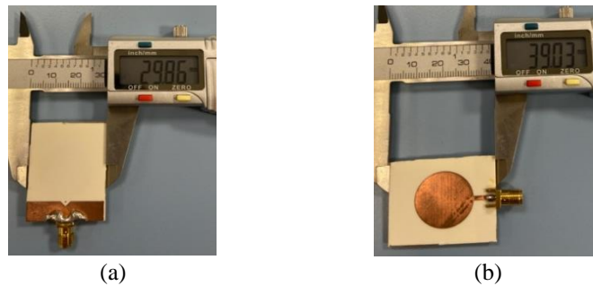
Figure 13. The dimension of the fabricated antenna (a) length and (b) width
