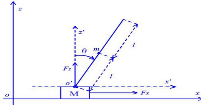
Figure 1. The Structure of the X-Z Inverted Pendulum
