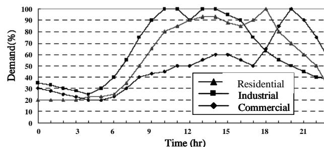
Figure 1. Daily Load Curves for the Three Load Types of the Microgrid
