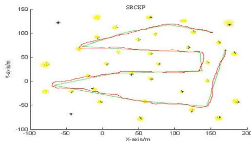
Figure 1. Results of SRCKF-SLAM (the green line is the true path, the red line is SLAM path, the black point is the real position of the landmark, the yellow point is the estimated position of the landmark)
