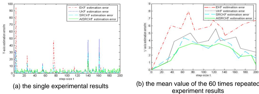
Figure 4. The SLAM Algorithm Error Comparison on the Y-axis under the Gaussian Noise
