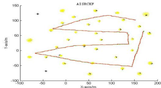
Figure 2. Results of AISRCKF-SLAM (the green line is the true path, the red line is SLAM path, the black point is the real position of the landmark, the yellow point is the estimated position of the landmark)
