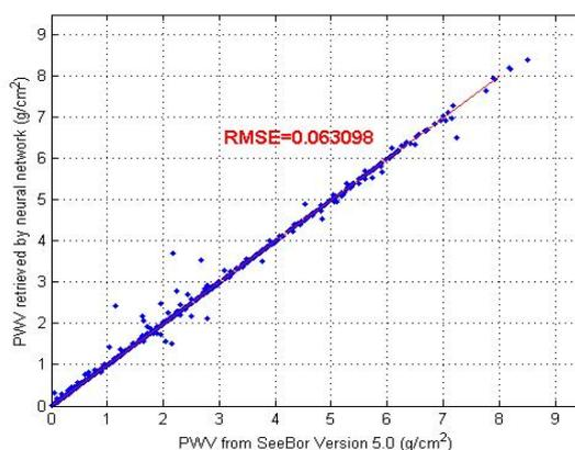
Figure 2. Comparison between the PWV Retrieved from Neural Network based on Algorithm and PWV from University of Wisconsin-Madison.
