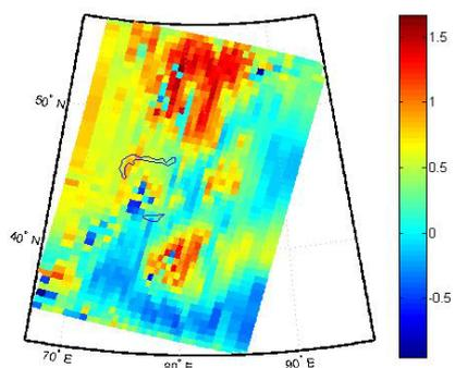
Figure 9. The Absolute Error of PWVs Retrieved by Neural Network and AIRS Product
