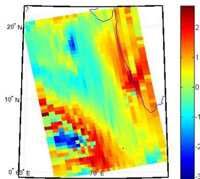
Figure 5. The Absolute Error of PWVs Retrieved by Neural Network and AIRS Product
