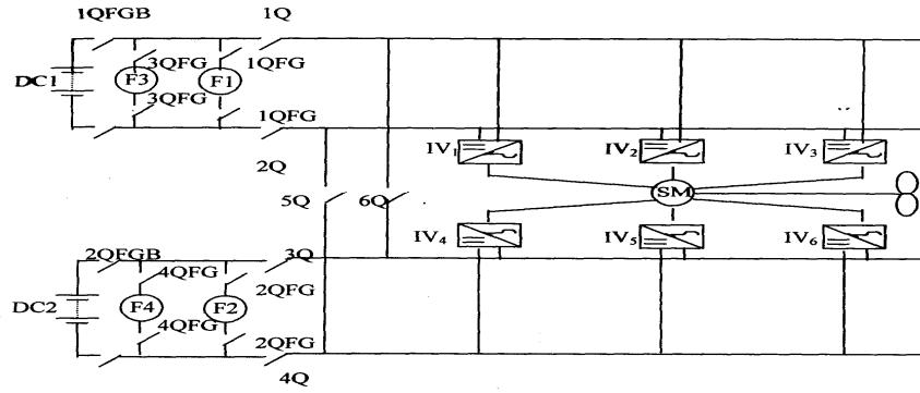
F<sub>1</sub>, F<sub>2</sub>—Diesel generator; F<sub>3</sub>, F<sub>4</sub>—Small Nuclear Power AIP Generator;
