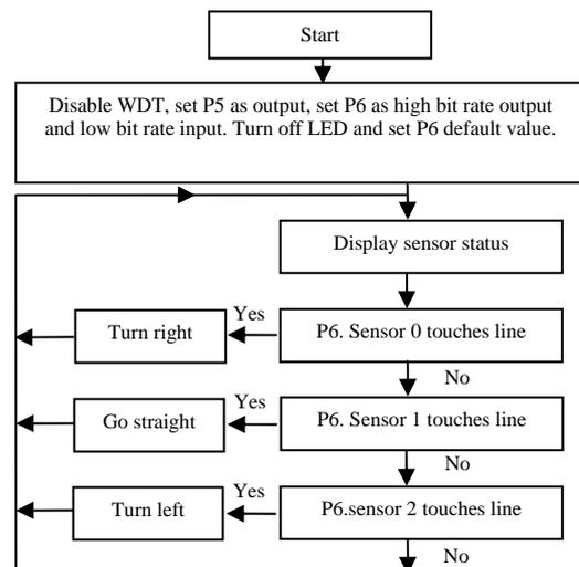
Figure 3. Optical Sensor Flow Chart
