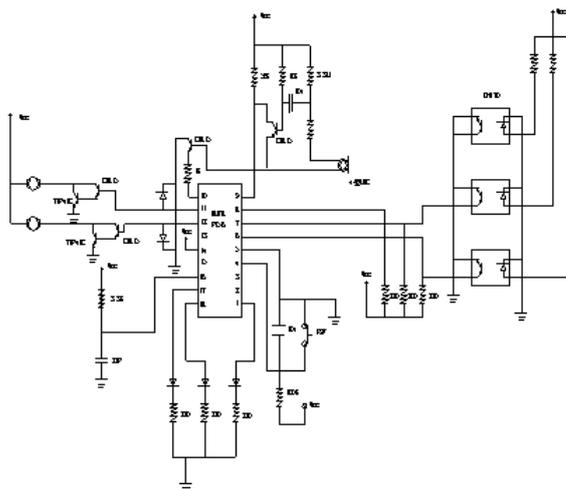
Figure 2. EM78447 Circuit Connection
