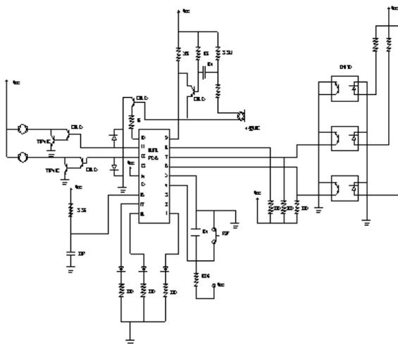
Figure 2. EM78447 Circuit Connection
