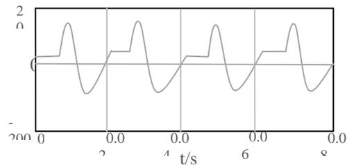
Figure 5. Simulation Waveform of Inrush Current
