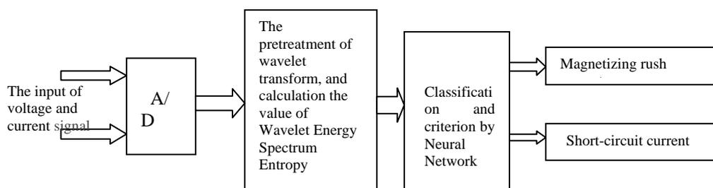
Figure 3. The Diagram of Identification Method of Inrush Current by Wavelet Energy Entropy Neural Network
