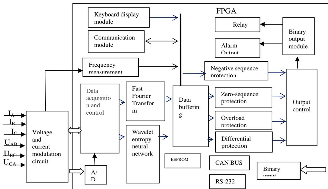
Figure 7. Hardware Design of Transformer Differential Protection based on FPGA
