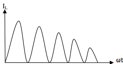
Figure 1. The Waveform of Inrush Current
