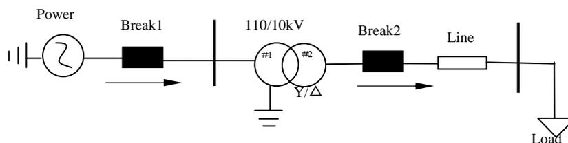
Figure 4. The Simulation Diagram of No-load Switching of Three-phase
