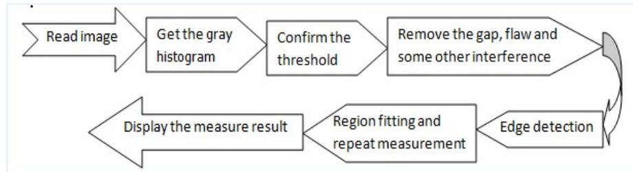
Figure1. Algorithm Process
