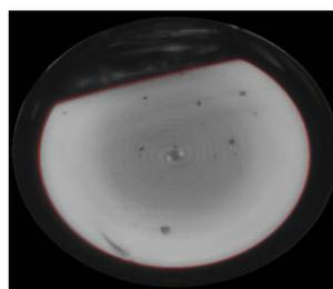
(b) Fiber core detection edge after screening
