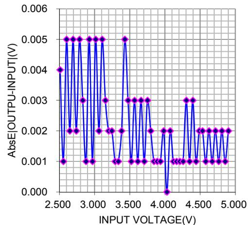
Figure 8. The Graph of the Absolute Error (AbsE) of the Measured Voltage Result at the Range of  $2.5\text{V}\sim 5\text{V}$
