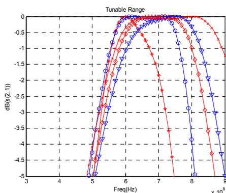
Figure 5. Insertion Loss (S21) of Matching Network
