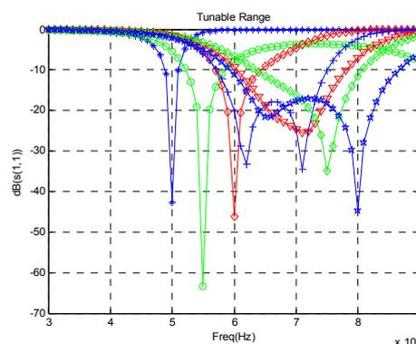
Figure 6. Return Loss (S11) of Matching Network
