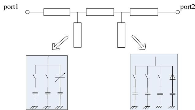
Figure 1. Structure of Tunable Impedance Matching Network
