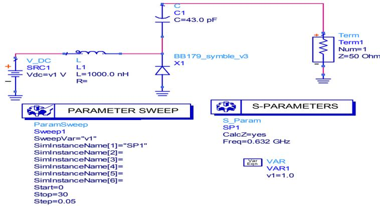
Figure 2. The Topology of Varactor Model
