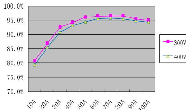
Figure 10. The Efficiency Curve of the Phase Shift Full Bridge Converter
