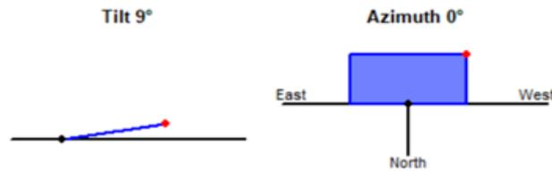
Figure 1. The depiction of the tilt angle and azimuth of solar panels
