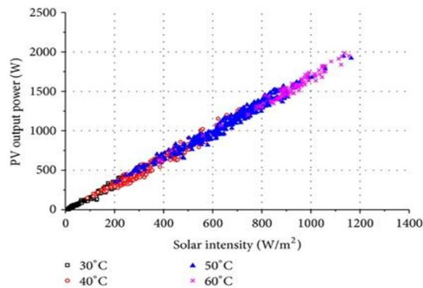
Figure 2. The effect of solar intensity on solar panel output power [15]
