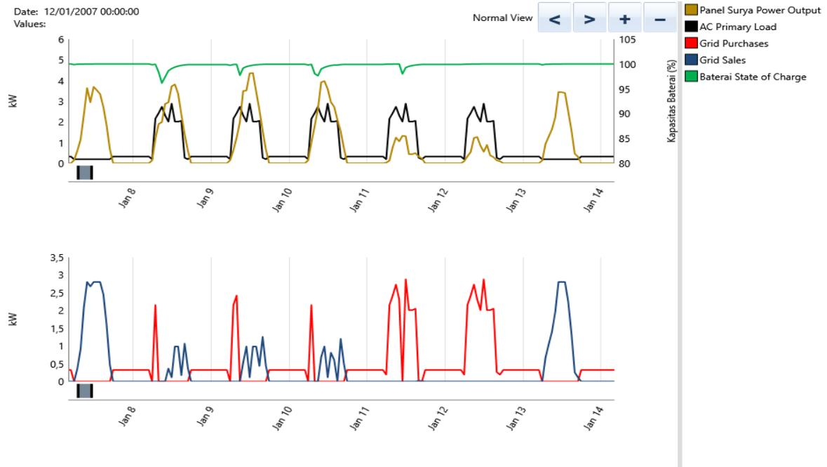
Figure 7. Graph of load power against solar panel output and battery (above) and energy export-import power graph (bottom)
