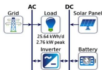
Figure 7. Hybrid system circuit diagram
