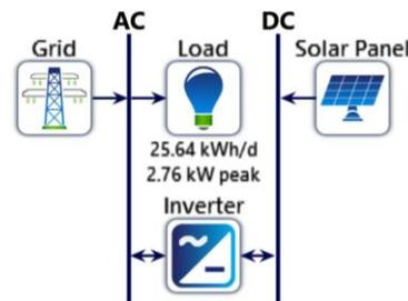
Figure 5. On-grid system circuit diagram
