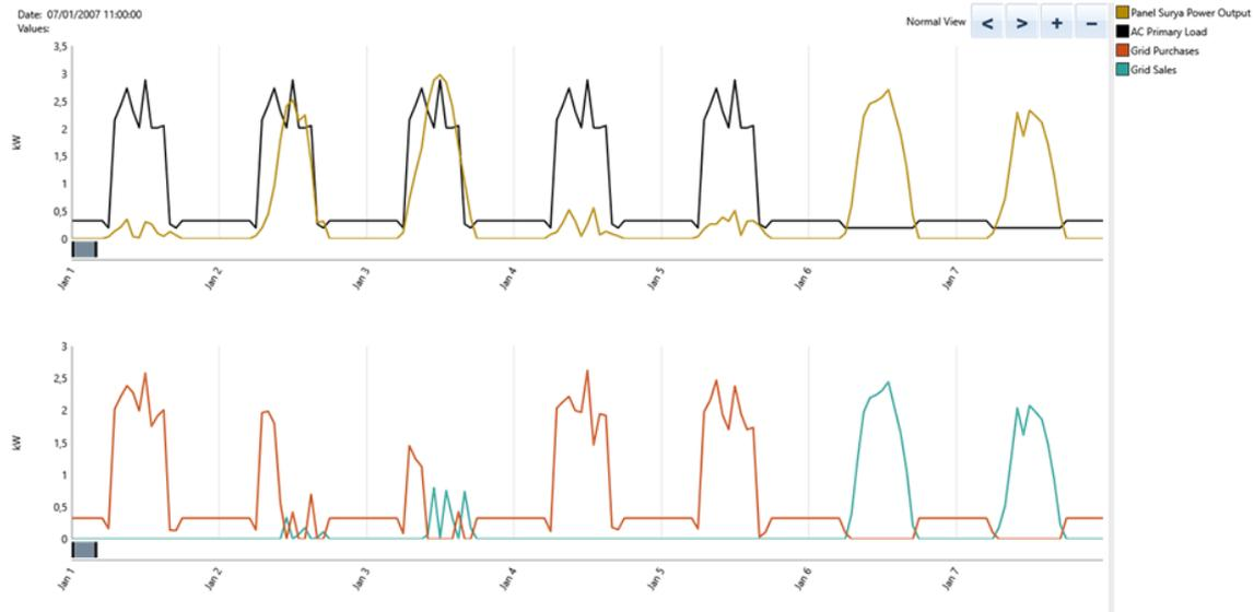
Figure 6. Graph of load power against solar panel output (above) and energy export-import power graph (bottom)
