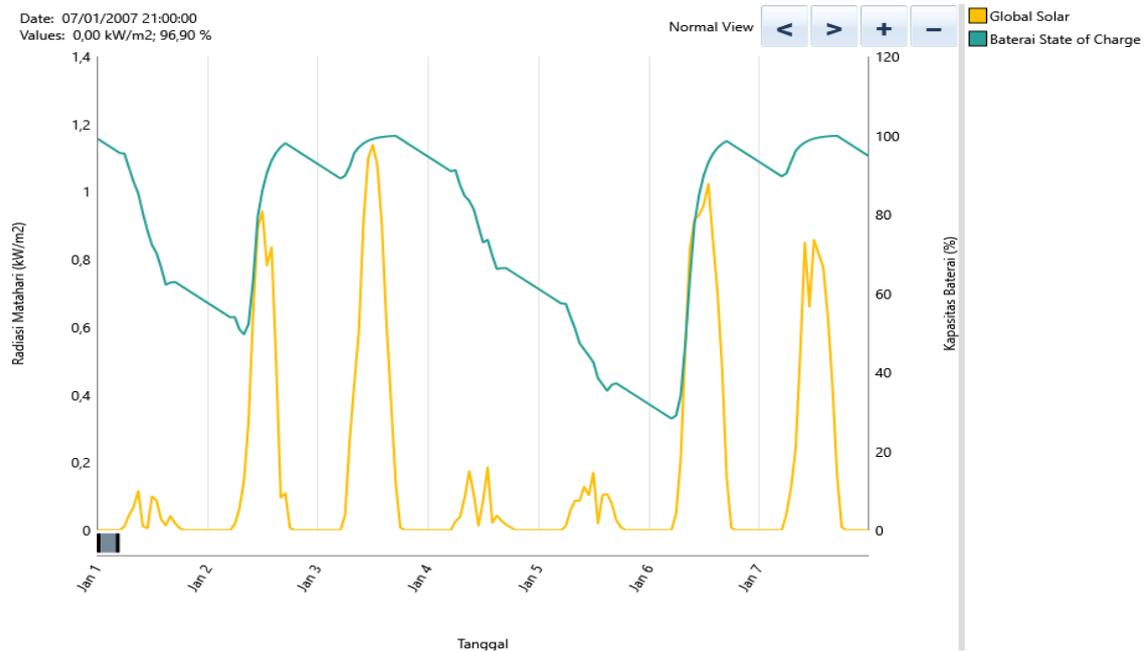
Figure 4. Graph of battery capacity against the solar intensity
