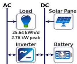
Figure 3. Off-grid system circuit diagram
