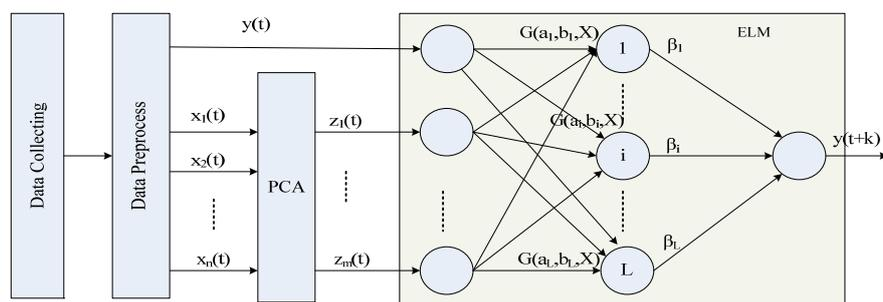
Figure 1. Software Aging Prediction Model
