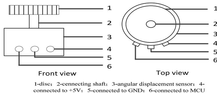
Figure 1(b). The Plan View and Top View of Sensor and Gear Connection
