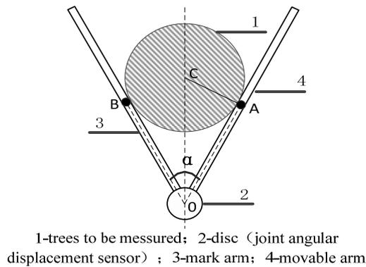
Figure 1(a). The Schematic Diagram of Diameter at Breast Height Measurement
