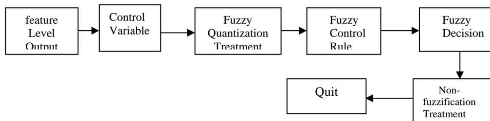
Figure 2. Fuzzy Reasoning System Schematic Diagram
