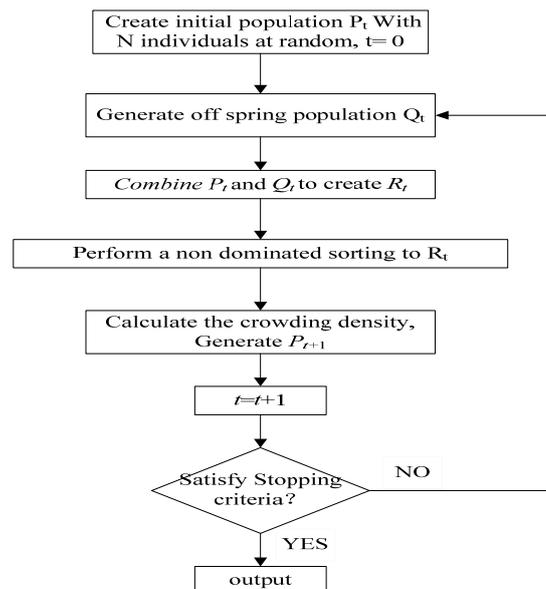
Figure 1. The Algorithm Flow of NSGA-II
