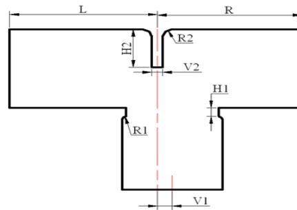
Figure 3. The Structure of the Power Divider
