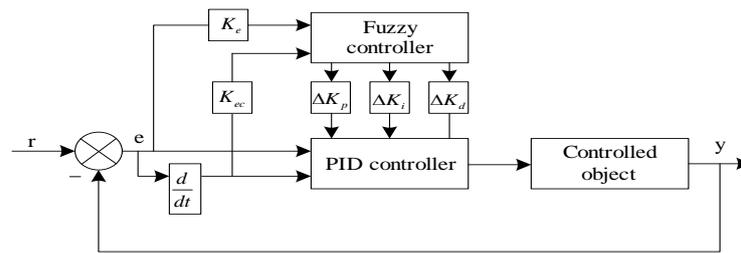
Figure 4. Control Structure of Fuzzy PID Control
