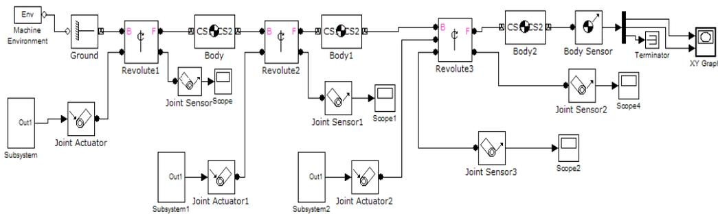
Figure 2. SimMechanics model of 3-DOF manipulator
