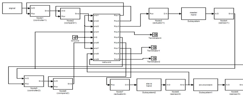
Figure 3. Simulation Diagram of Tele-operation Manipulators System based on TrueTime
