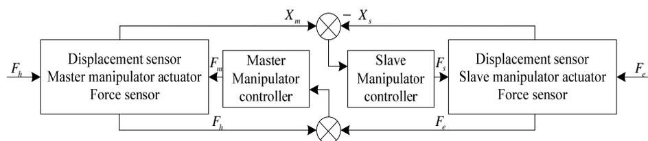
Figure 1. Bilateral servo control architecture with force deviation feedback
