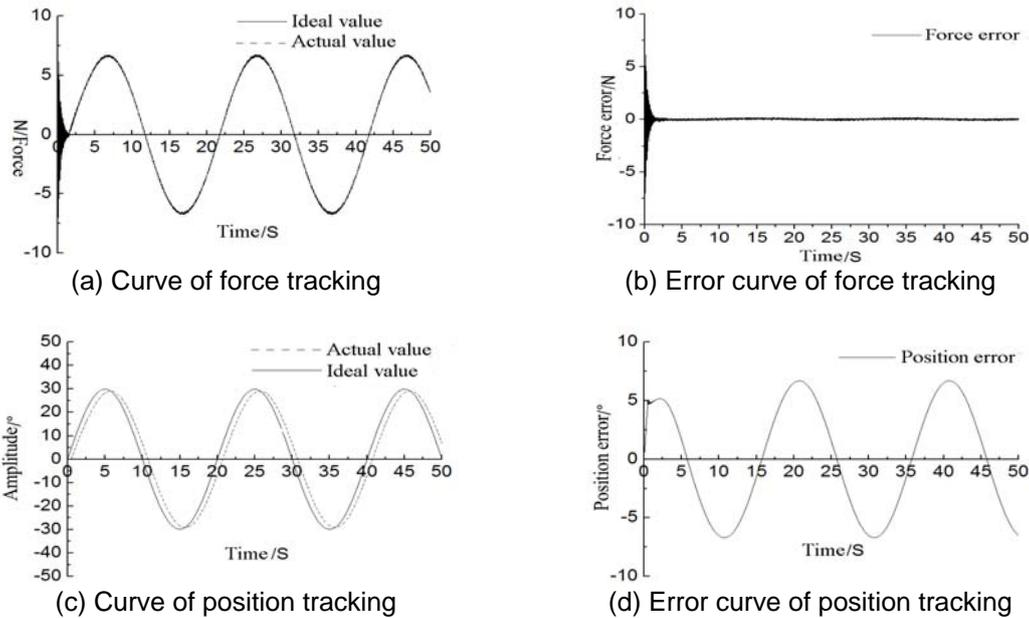
Figure 7. Simulation Results of Fuzzy PID Control Method
