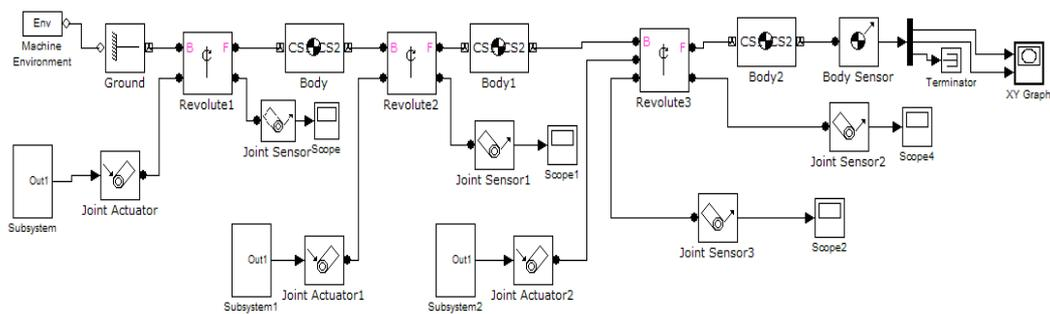
Figure 2. SimMechanics model of 3-DOF manipulator
