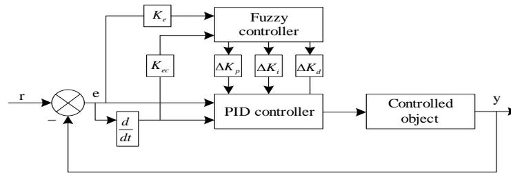
Figure 4. Control Structure of Fuzzy PID Control
