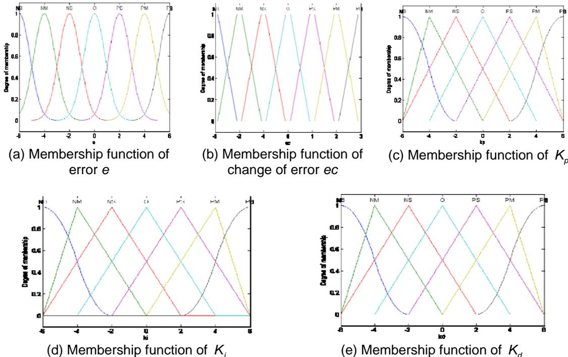
Figure 5. Curves of Membership Function of  $e$ ,  $ec$ ,  $\Delta K_p$ ,  $\Delta K_i$  and  $\Delta K_d$
