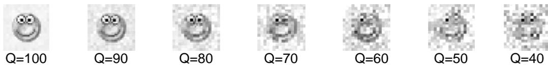
Figure 5. Watermark Extraction Image under Different JPEG Compression Ratio (Q represents the compression ratio)
