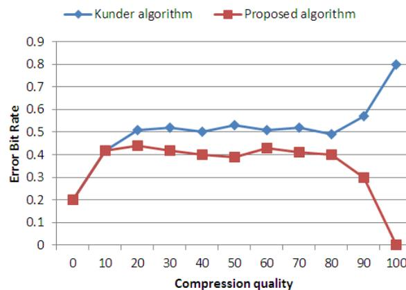
Figure 8. Comparison of Extracted Watermark BER after JPEG Compression
