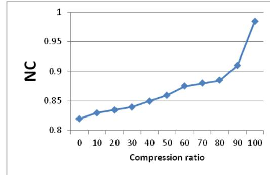
Figure 7. The Values of NC after JPEG Compression Attack
