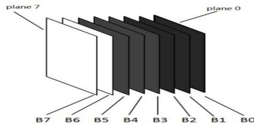
Figure 2. Schematic Diagram of Bit Plane Decomposition
