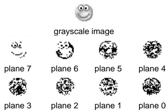
Figure 3. Watermark Image Each Bit-plane after Decomposition
