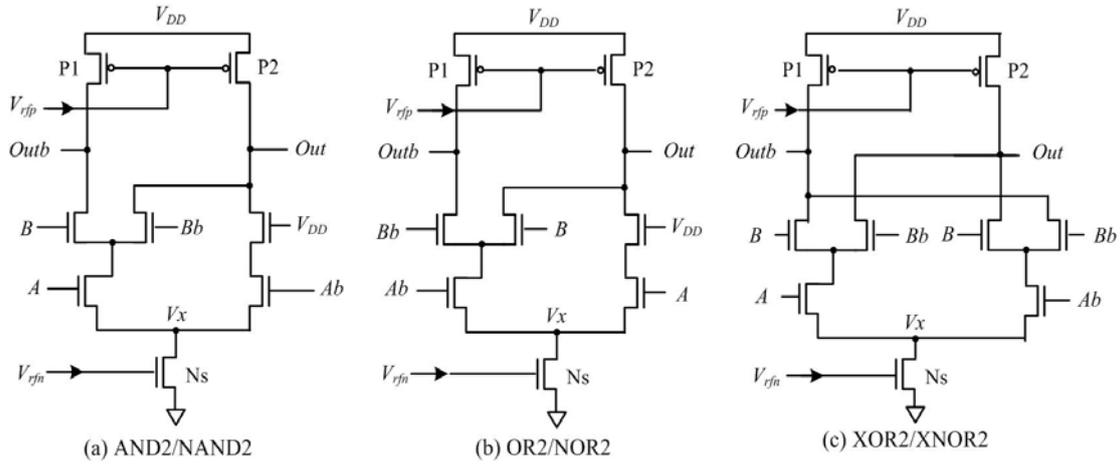
Figure 2. Basic gates based on MCML
