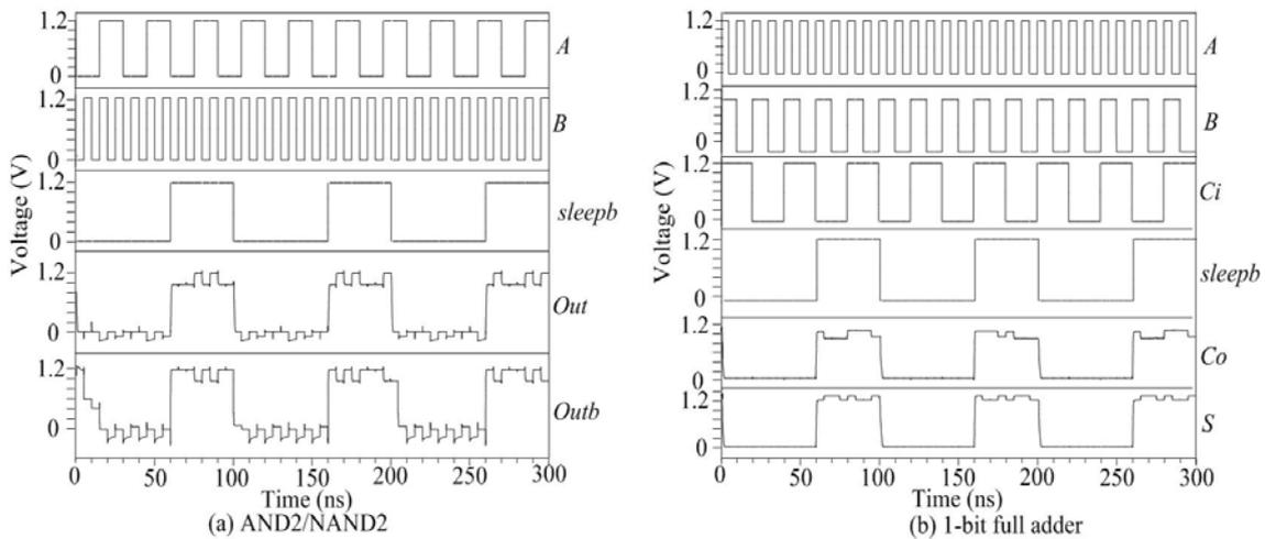
Figure 8. Simulation waveforms of the AND2/NAND2 and 1-bit full adder based on power-gating MCML
