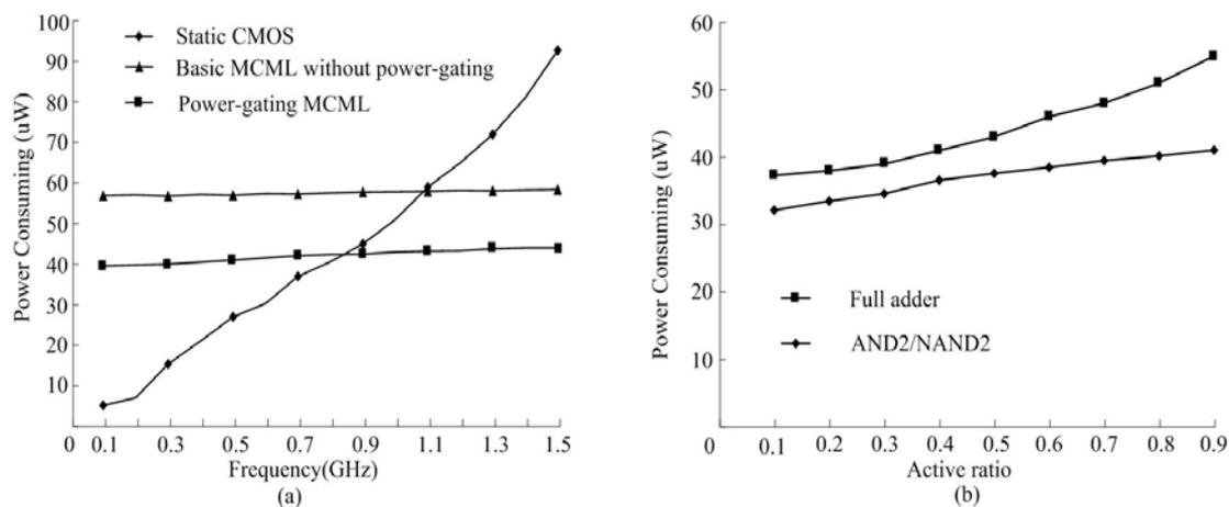
Figure 10. (a) Power consuming comparisons among the 1-bit full adders based on the power-gating MCML, static CMOS, and basic MCML without power-gating, and (b) Power dissipation of power-gating circuits with various active ratio
