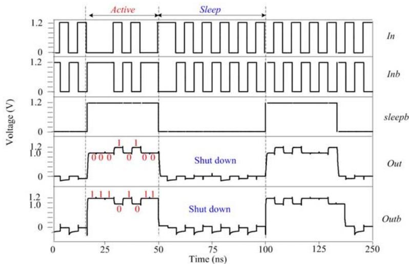
Figure 6. Simulated waveforms for the power-gating MCML inverter/buffer
