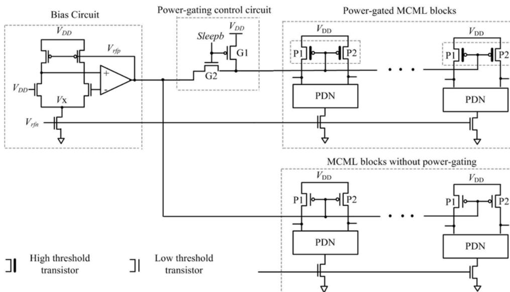
Figure 7. The power-gating realization for both MCML block without power-gating and power-gated MCML block
