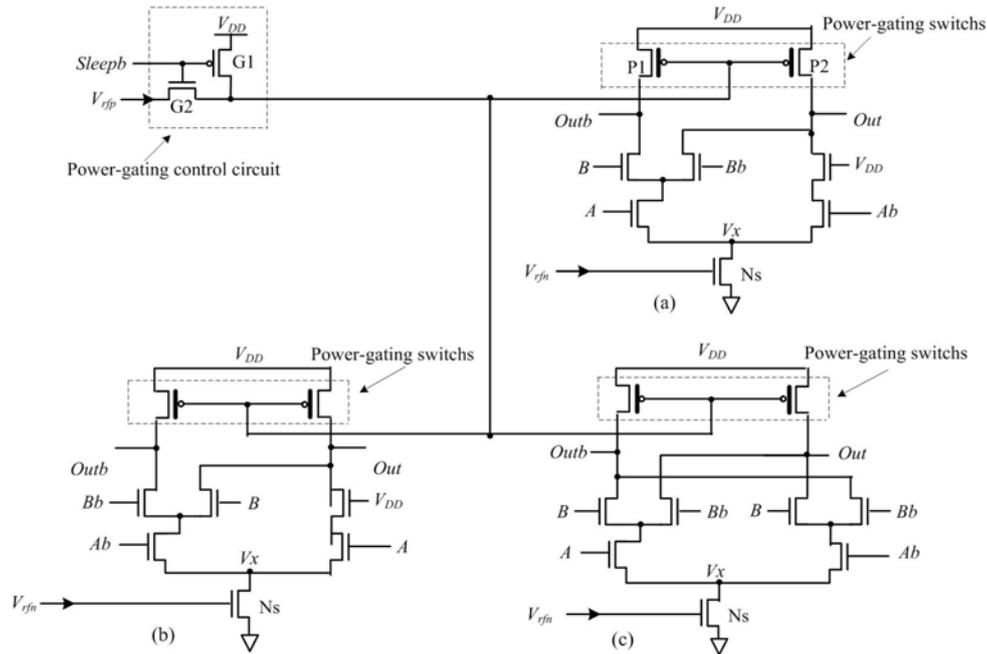
Figure 5. Power-gating MCML gates. (a) AND2/NAND2, (b) OR2/NOR2, and (c) XOR2/XNOR2
