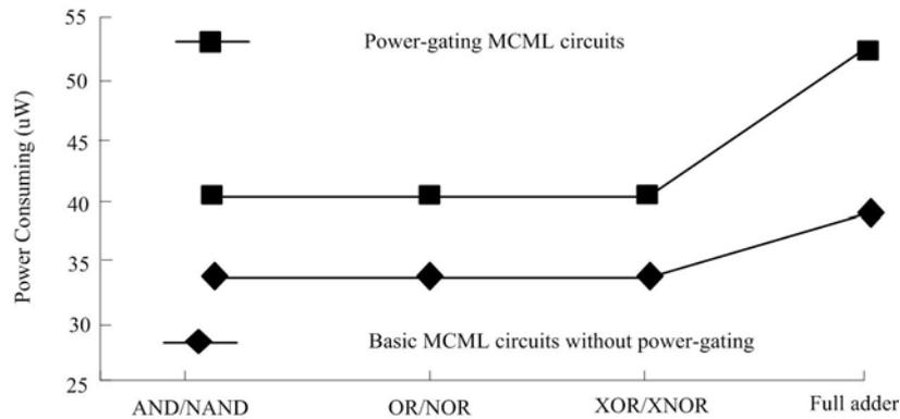
Figure 9. Power dissipation comparisons of the basic gates and 1-bit full adder between the power-gating MCML and convention MCML without power-gating
