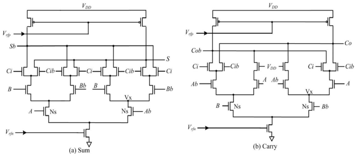
Figure 3. 1-bit Full adder based on MCML
