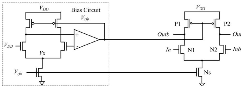
Figure 1. MCML inverter/buffer and its bias circuit
