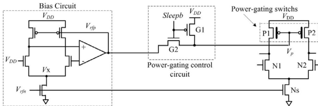
Figure 4. Power-gating scheme for MCML circuits
