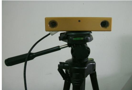
Figure 3. Binocular vision system
