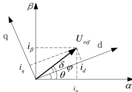
Figure 3. Position of Uref in  $\alpha$ - $\beta$  frame and d-q frame
