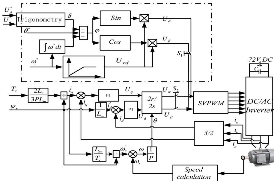
Figure 4. Rotor field-oriented vector control switching into constant V/F based on SVPWM with the phase angle compensation
