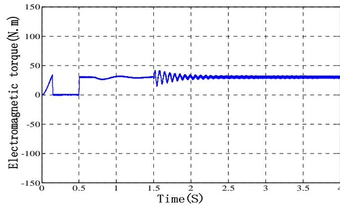
Figure 8. Torque curve of rotor field-oriented control switch into the open-loop constant V/F control with the phase angle compensation
