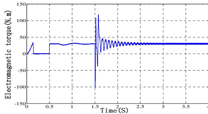
Figure 5. Torque curve of rotor field-oriented control switch into the open-loop constant V/F control
