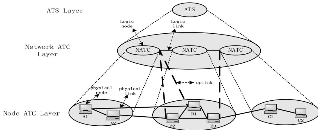
Figure 5. The configuration of Network ATC Layer
