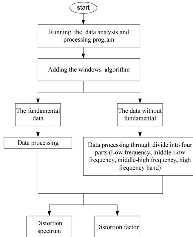
Figure 3. Flow chart of the data analyzing and processing program
