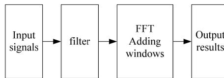
Figure 2. Structure chart of the data processing in frequency band
