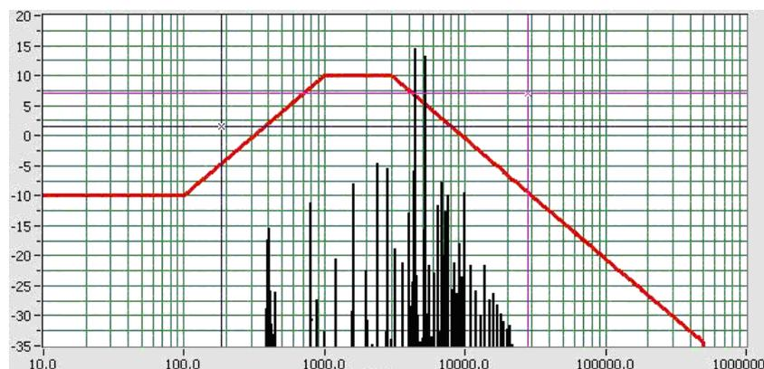
Figure 6. The AC voltage distortion spectrum chart
