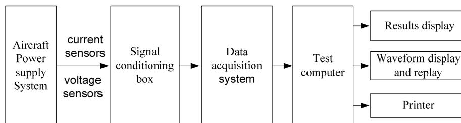
Figure 4. The structure chart of test system
