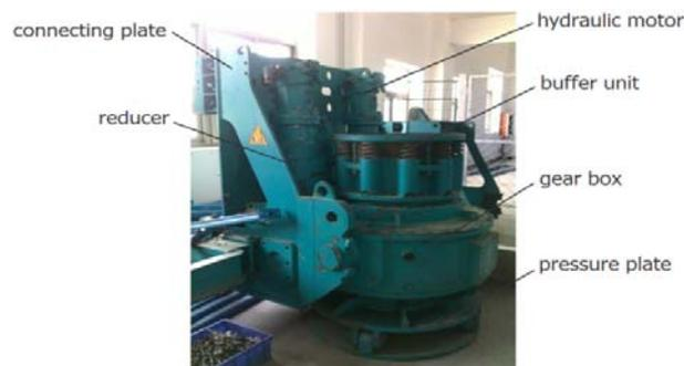
Figure 1. Power head structure
