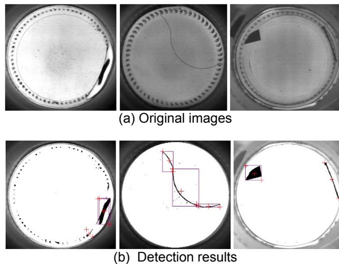
Figure 6. The defect detection of bottle bottom
