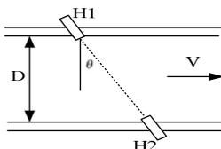
Figure 1. The Basic Principle of Ultrasonic Flow Meter
