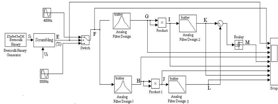
Figure 6. The Architecture of FSK Simulation System in MATLAB/SIMULINK
