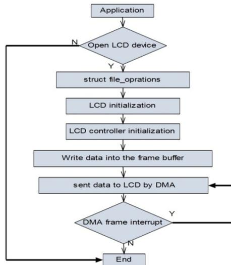
Figure 3. Monochrome LCD Program Structure based on Framebuffer
