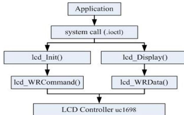
Figure 2. The Program Structure based on GPIO
