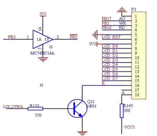
Figure 1. LCD External Interface Circuit
