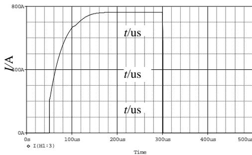
Figure 5. Turn Off Process Waveform of Anode-cathode Current
