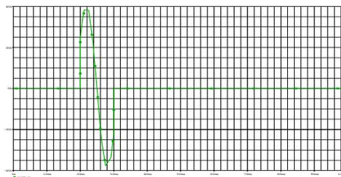
Figure 20. Current Waveform of IGCT
