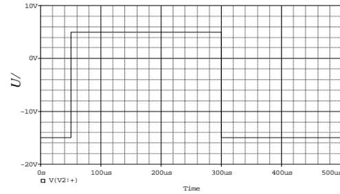
Figure 4. Turn Off Process Waveform of Grid Voltage
