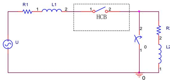
Figure 14. Equivalent Short Circuit
