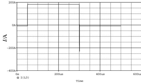
Figure 3. Turn Off Process Waveform of Grid Current
