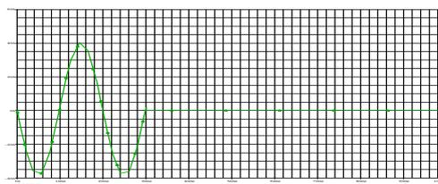
Figure 17. Current Waveform of IGCT
