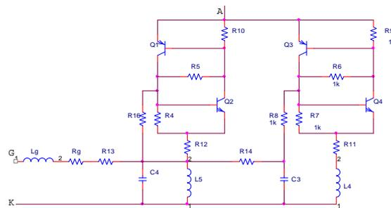
Figure 1. Electricity Model of IGCT
