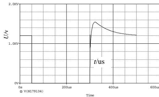
Figure 6. Turn Off Process Waveform of Anode-cathode Voltage
