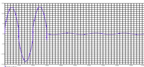
Figure 15. Voltage Waveform of both sides Mechanical Switch
