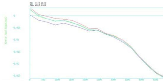
Figure 15. X-axis Straightness Error in XZ Plan
