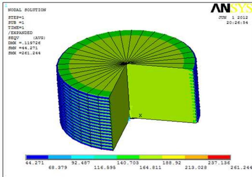
Figure 7. The von mises stress nephogram in the preload condition (simple stretching)
