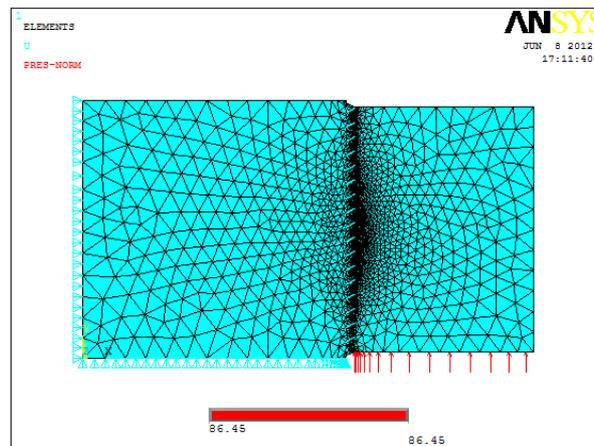
Figure 5. The axisymmetric finite element model
