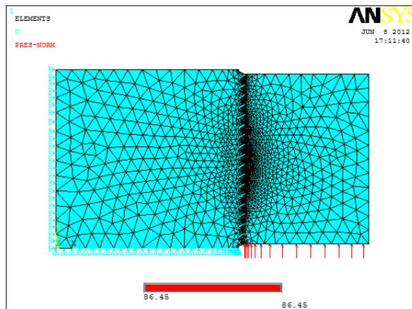
Figure 5. The axisymmetric finite element model
