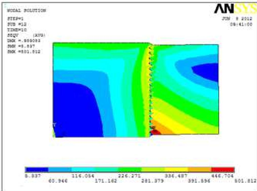
Figure 9. The von mises stress nephogram in the preload condition (contact analysis)
