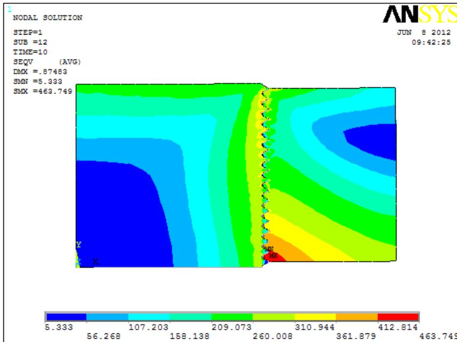
Figure 11. The von mises stress nephogram in the work condition (contact analysis)
