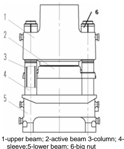
Figure 1. Schematic diagram of PRESS
