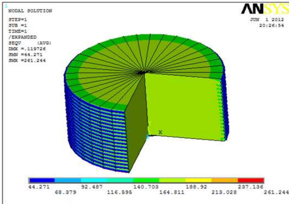
Figure 8. The von mises stress nephogram in the work condition (simple stretching)
