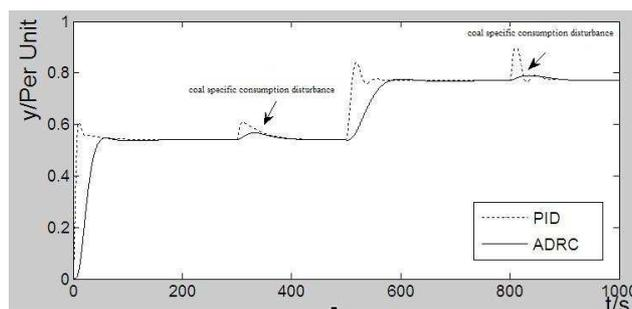
Figure 6. Curves of intermediate point temperature's emulation due to feedwater disturbance and fuel disturbance at 50%~75% BMCR
