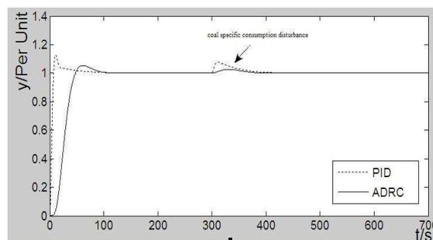
Figure 5. Curves of intermediate point temperature's emulation due to feedwater disturbance and fuel disturbance at 50% BMCR
