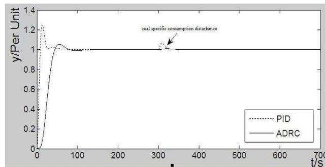
Figure 3. Curves of intermediate point temperature's emulation due to feedwater disturbance and fuel disturbance at BMCR
