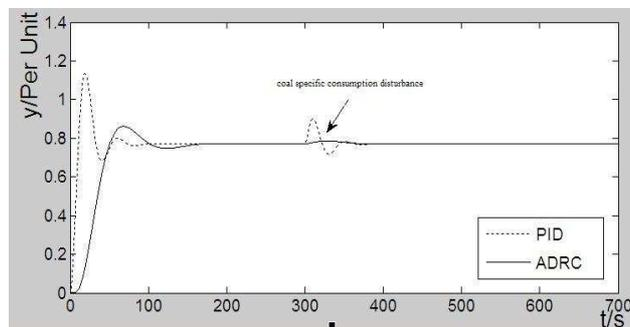
Figure 4. Curves of intermediate point temperature's emulation due to feedwater disturbance and fuel disturbance at 75% BMCR
