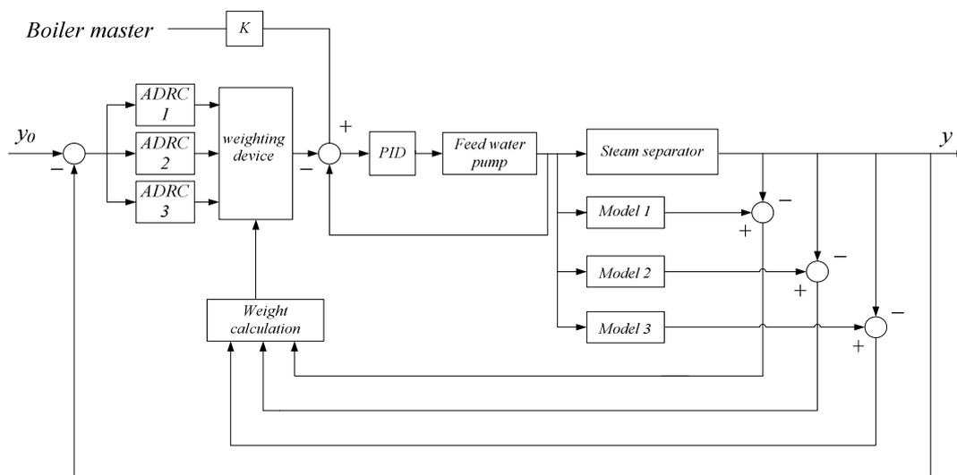
Figure 1. Structure of Multi-model Control System Based on ADRC
