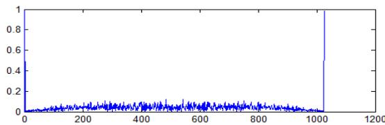
Figure 10. The spectrum of the bitsream of sigma-delta output
