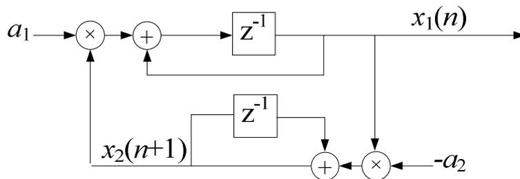
Figure 2. The structure of the numerical resonator
