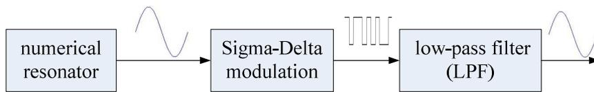
Figure 1. The scheme of the sinusoidal signal generator
