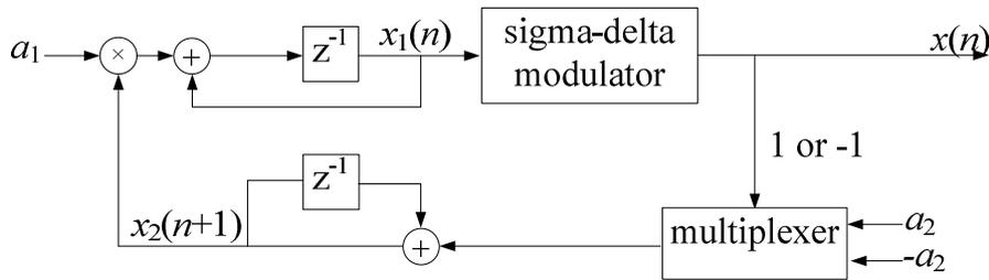
Figure 4. The modified resonator
