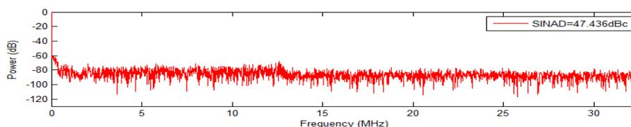
Figure 12. The spectrum of ADC response
