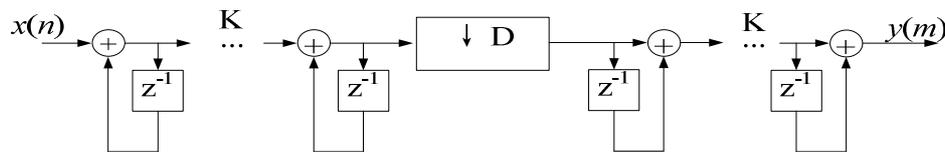
Figure 6. The structure of  $k$  CIC filter
