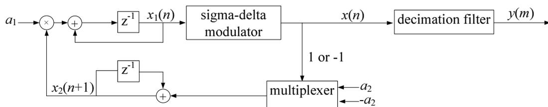
Figure 7. The structure of sigma-delta modulation based sinusoidal signal generator
