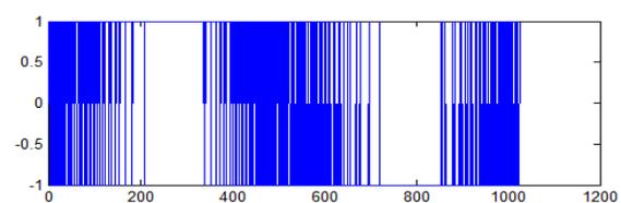
Figure 9. The bitsream of sigma-delta output
