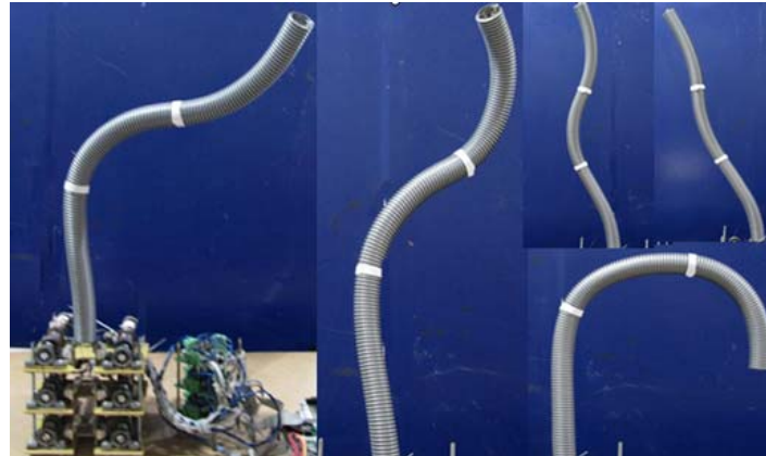
Figure 7. Space motion experiment the robot with three sections
