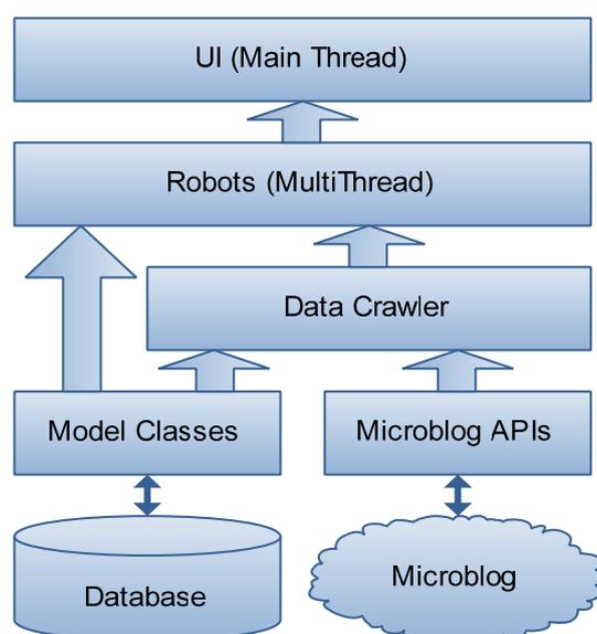
Figure 1. Basic Structure of MBCrawler
