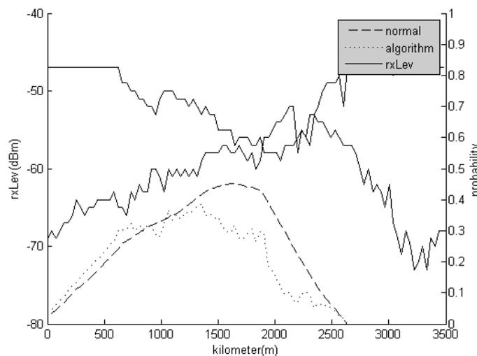
Figure 9. Probabilities of interference of normal transmission and transmission method
