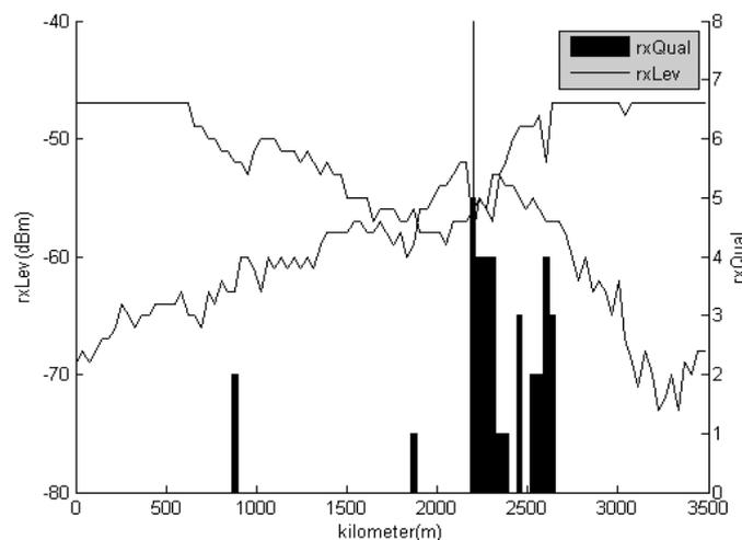
Figure 6. rxLevs and rxQuals of two cells
