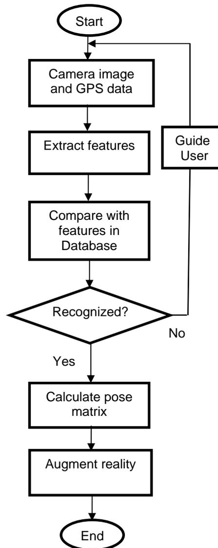
Figure 3. Conceptual diagram of proposed framework
