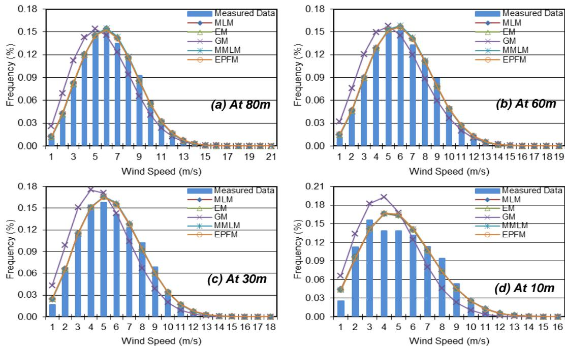
Figure 4. Weibull probability distributions of wind speeds at four heights at Hawksbay
