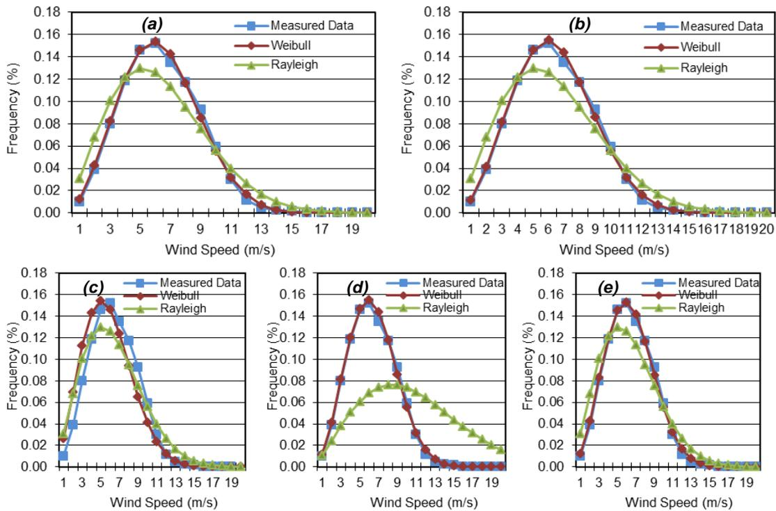
Figure 5. Comparison of Weibull & Rayleigh distribution with measured wind data at 80m height using (a) MLM; (b) EM; (c) GM; (d) MMLM; and (e) EPFM
