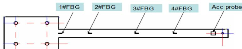
Figure 6. The Cantilever Beam and FBG
