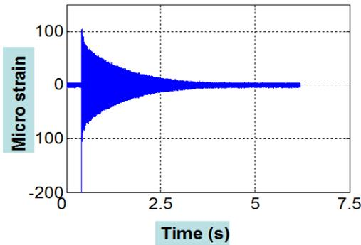
Figure 8. Impact signal of Cantilever Beam
