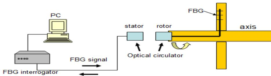
Figure 2. Experimental Set-Up for Dynamic Strain Detection by FBG
