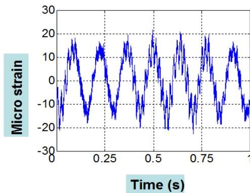
Figure 10. The Rotating Cantilever Beam Dynamic Strain Data From 1#FBG in 420RPM
