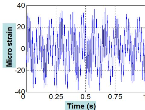
Figure 10. The Rotating Cantilever Beam Dynamic Strain Data From 1#FBG in 655RPM
