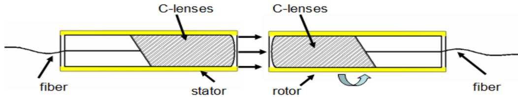
Figure 1. Working Principle for Rotary Optic Signal Transmission
