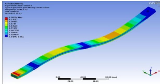
Figure 5. The 3<sup>rd</sup> Strain Mode Shape
