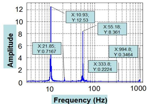
Figure 11. The Rotating Cantilever Beam Dynamic Strain From 1# FBG in frequency domain in 655RPM
