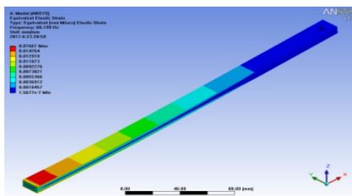
Figure 3. The 1<sup>st</sup> Strain Mode Shape
