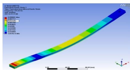
Figure 4. The 2<sup>nd</sup> Strain Mode Shape
