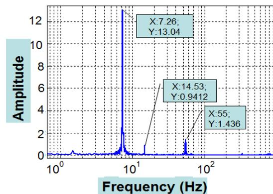
Figure 11. The Rotating Cantilever Beam Dynamic Strain From 1# FBG in Frequency Domain in 420 RPM
