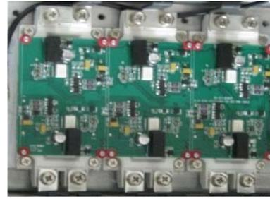
Figure 2. IGBT and Radiator Assembly
