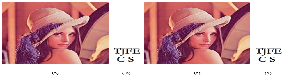
Figure 4. Host Image (a), Watermark (b), Watermarked image (c), Extracted watermark (d) (PNSR = 29.64, NC = 0.9986)
