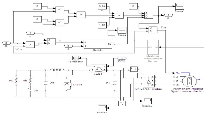
Figure 2. MPPT Simulation Module of Wind Power Generation System
