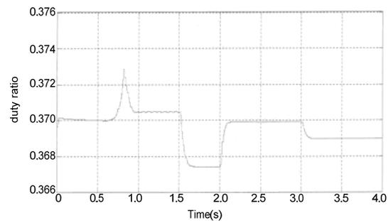
Figure 4. The Change of Control Signal (duty ratio) Versus Wind Speed
