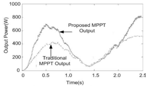
Figure 5. MPPT Output by using Proposed Method Compare with by using Traditional Method
