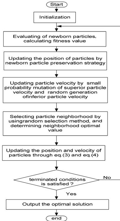
Figure 1. MPPT Control Algorithm based on Improved Particle Swarm Optimization
