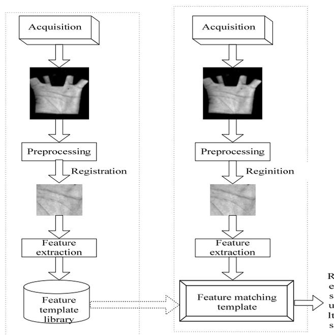
Figure 1. Structural Diagram of Palmprint Recognition System
